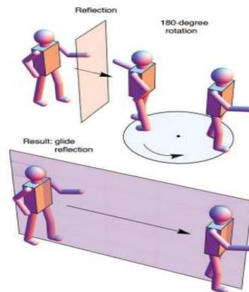
Figure 2. Composing a mirror reflection with a rotation yields a glide reflection.
