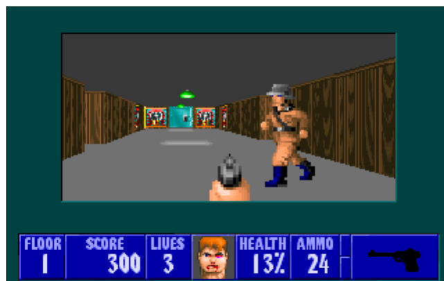
Fig. 3: Wolfenstein 3D uses ray casting to implement a 3D perspective while using 2D sprites for most other entities, like enemy characters.
