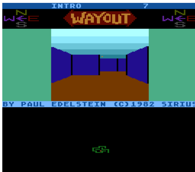
Fig. 7: Screenshot of WayOut running on an Atari 800, showcasing the simplistic solid-color walls used in this game's ray casting engine.
